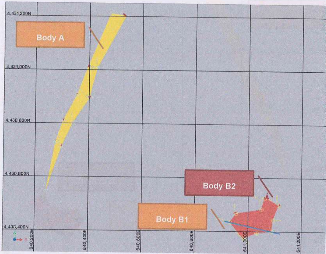
Figure 35. Location of the three mineralized bodies A, B1 and B2 modelled; blue full line is location of cross section (see Figure 36).
