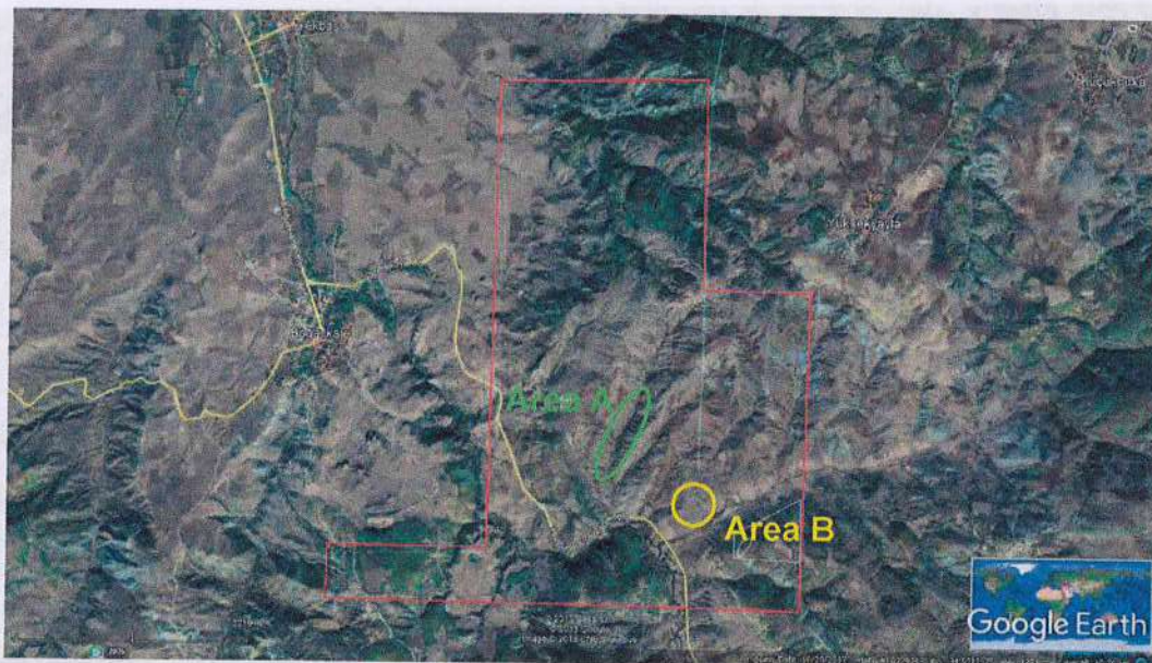
Figure 4. The licence area 200712071 (red line) is located appr. 6 km to the E of the village Bogazkale; areas of drilling activities in green and yellow circle, Area A has sulfidic mineralization starting from some meters below surface, Area B has oxidized mineralization starting directly at surface and sulfidic mineralization below. (Source: Google Maps).
