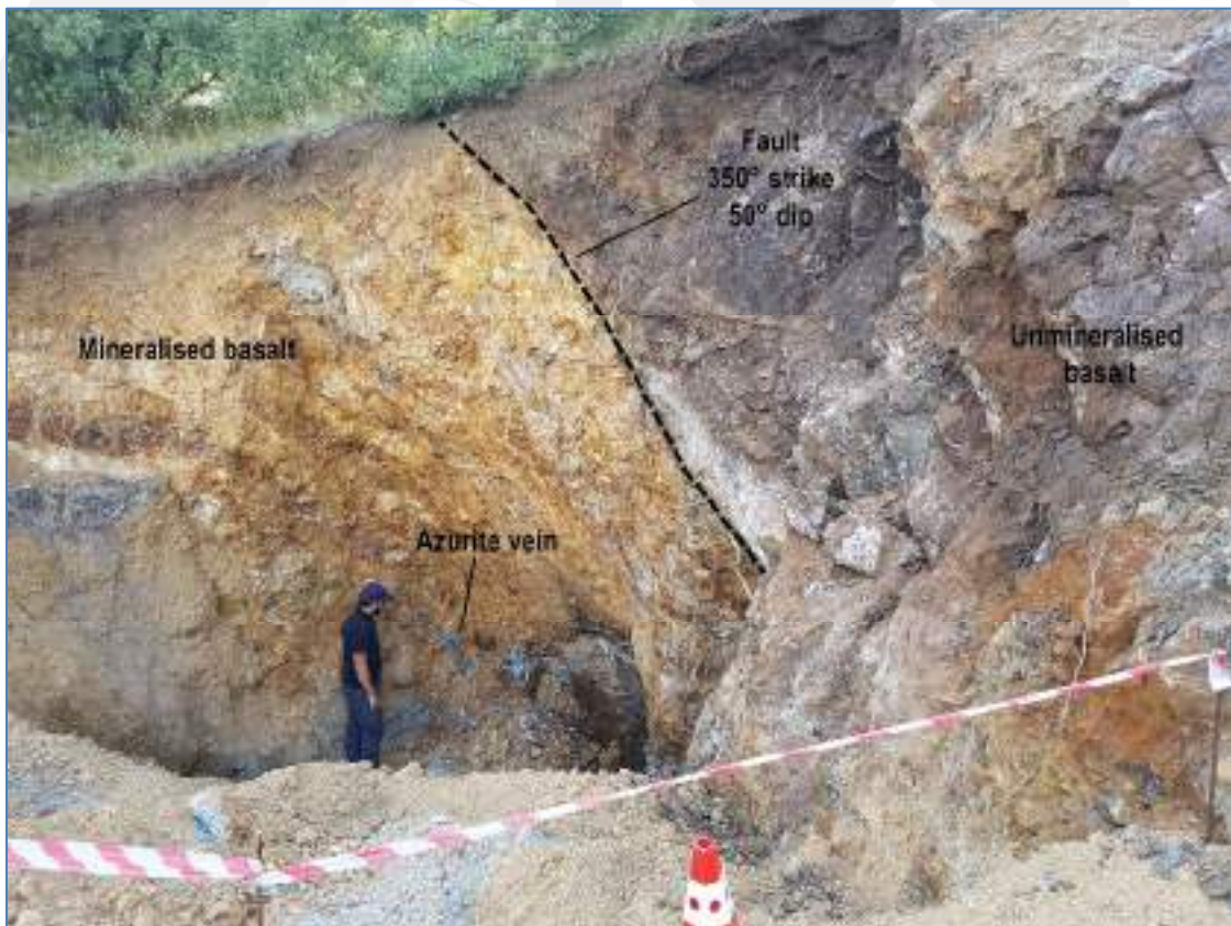
Figure 14: Area B. Looking north. Photo shows mineralised basalt with azurite veining and post mineralisation faulting.
