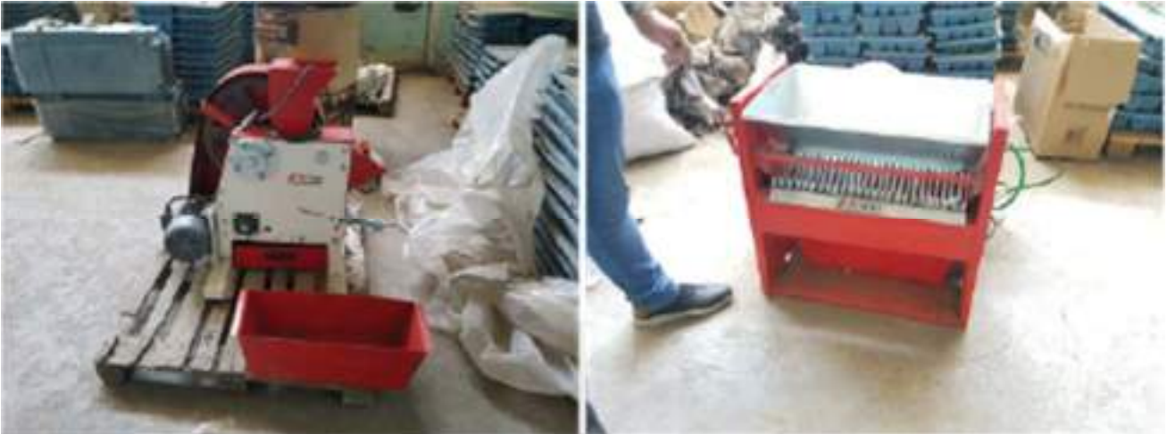
Figure 21: First split equipment used by AVOD: jaw crusher (left) and aggregate splitter (right).
