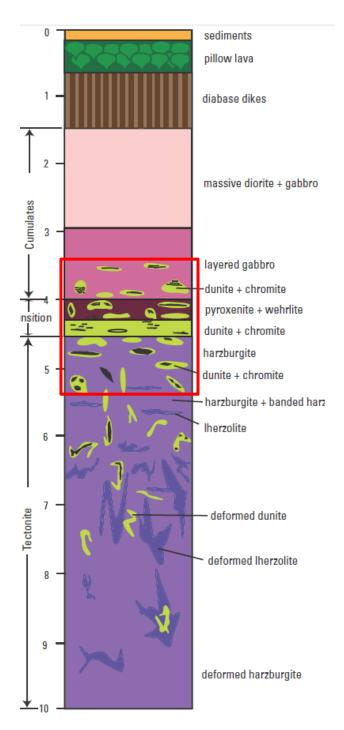
Figure 13. Typical lithological column of an ophiolite sequence (source: USGS). The red square indicates the interpreted stratigraphic position of the lithologies of interest in license 200712070.
