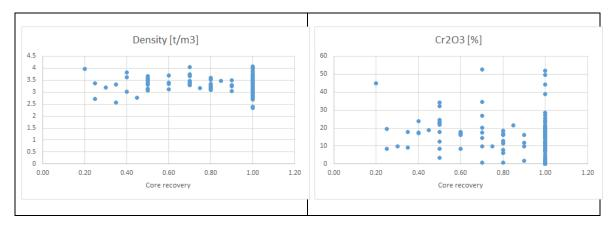
Figure 18. Cross plots of bulk density and Cr<sub>2</sub>O<sub>3</sub> vs. core recovery.
