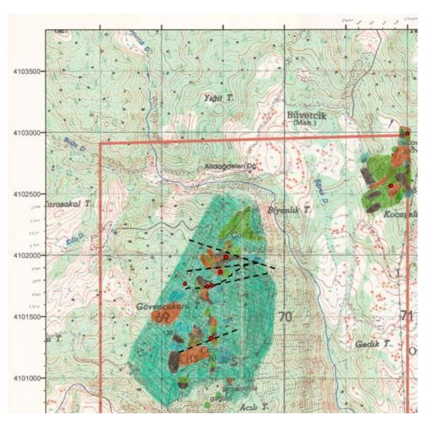
Figure 11: Results of the geological mapping (chromite - red dots and probable faults - dashed lines).
