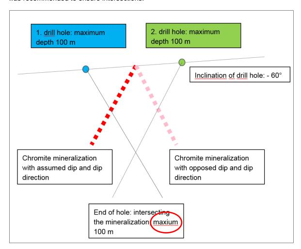
Figure 14. Proposed scheme of exploration drilling.
