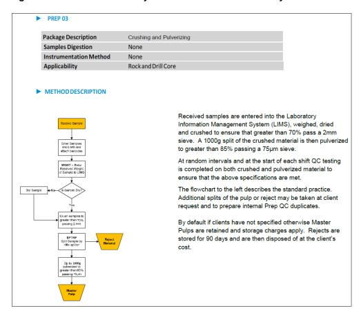
Figure 16. PREP03 - sample preparation as described by ARGETEST.
