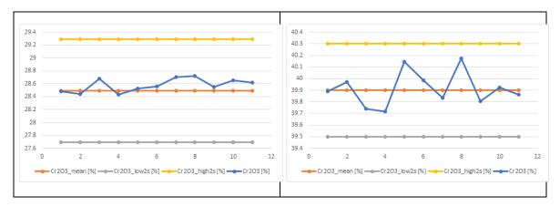
Figure 19. Assay results for CRMs AMIS 0387 (left) and AMIS 0388 (right) for Cr<sub>2</sub>O<sub>3</sub>.
