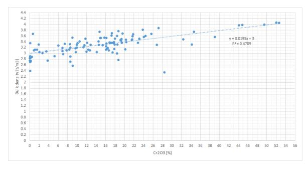
Figure 20. Cross plot bulk density [t/m³] vs. Cr<sub>2</sub>O<sub>3</sub> [%] showing a high scatter.
